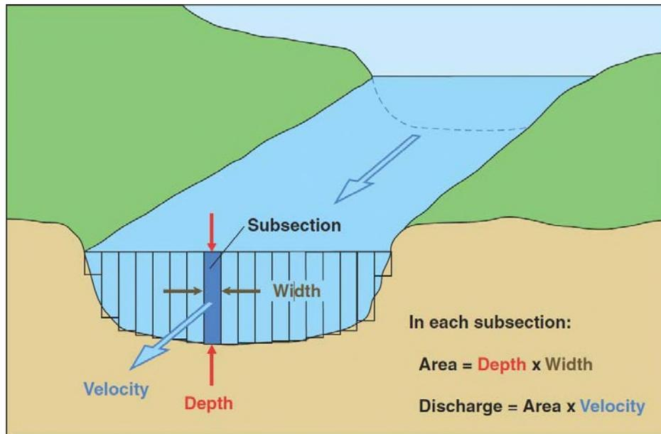
The stream cross section (transect) is divided into units of width (subsections) and the velocity and depth are measured at each. Discharge (area of a single subsection times the velocity measured) is calculated for each subsection. The resulting values are summed to obtain the instantaneous discharge for the stream at that transect.
